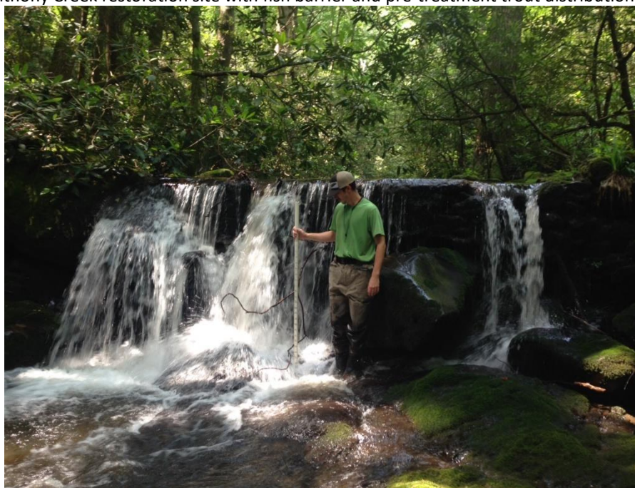
Figure 2: Measuring the height of the mill dam fish barrier for the Anthony Creek Restoration Project.
