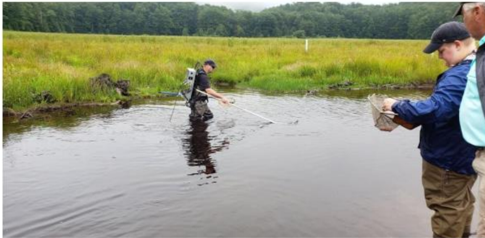
Figure 6 Electroshock sampling of South Branch Bowman Creek in project area July 22, 2019.
